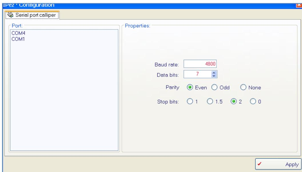
It should be stressed that if the calliper is not always connected to the same COM port, the port connection will have to be specified each time for the calliper to function.
